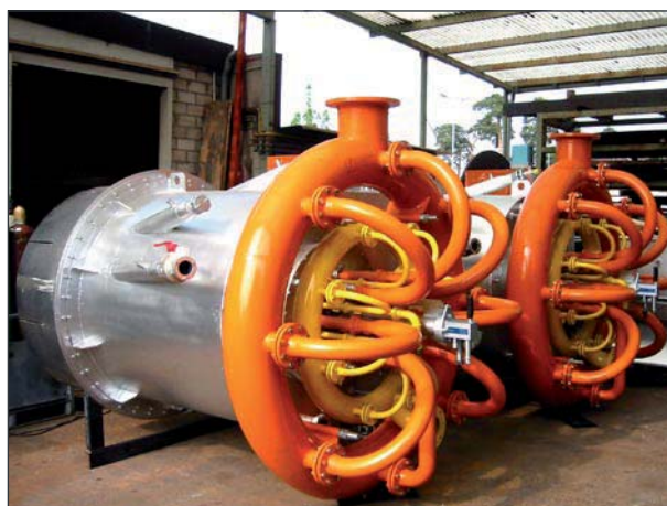
Fig.3 : PILLARD “GRC LONOXFLAM” burner seen from the rear
