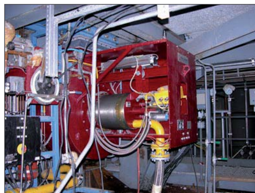
Fig.6 : PILLARD "GROOM" burner Brescia plant (Italy)
