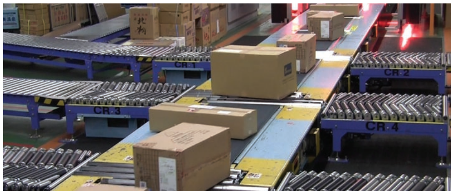
Above: The slide sorter also handles non-conveyable items Left: The diverting sorter unit
