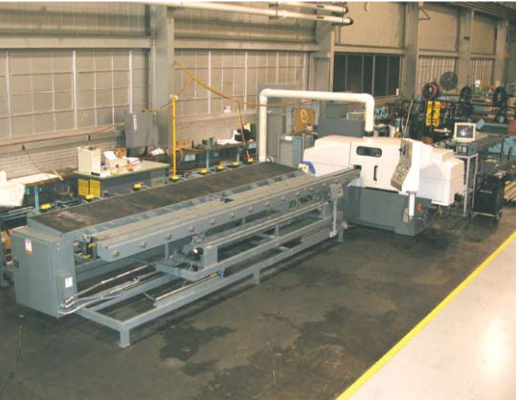
An automated infeed table facilitates the automatic operation of the grinder by supporting and feeding bars as they are ground.
