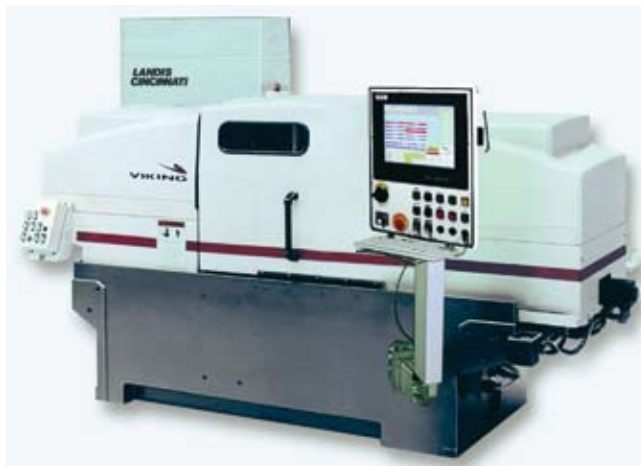
The Landis Cincinnati Viking Super Series II centerless grinder automatically grinds bar stock using a through-feed grinding cycle.
