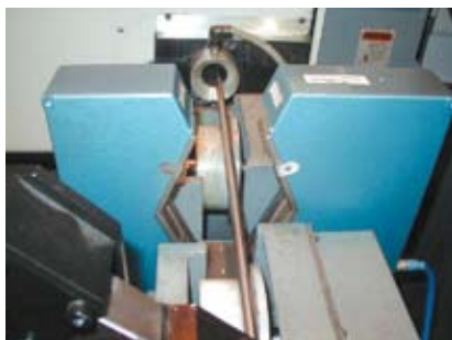
The outfeed table rollers turn faster to unload the bars at the same rate or a faster one than the rate that they are ground.
