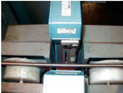
A laser gage system controls automatic operation of the feeding automation and the centerless grinder.
