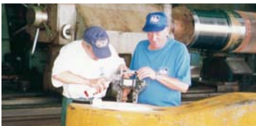
Magnetic-particle inspection before pre-machining and welding
