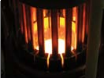
Cold crucible Melting with a CELES MP100 inverter
