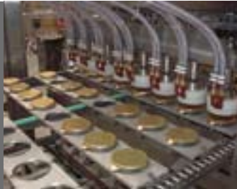
Induction cap sealing with a CELES MP75 inverter
