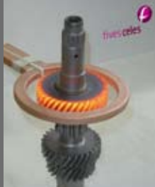
Example of gear heating
