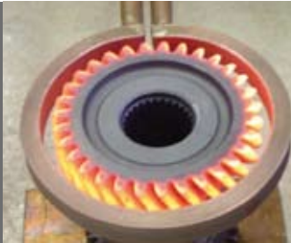
Example of gear heating
